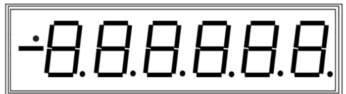
Front view of BDF units made with 4 and 6 digits. Location of the digits, negative sign, and decimal points.
